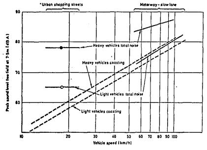
Figure 5-8. Total Vehicle Noise and Coasting Noise Source: (5-17)
